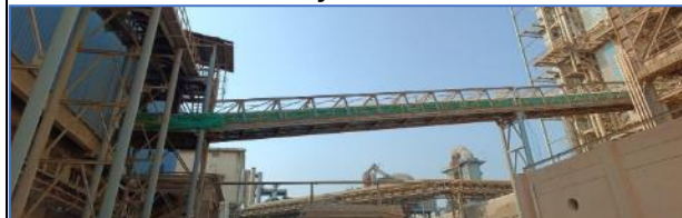
Closed conveyor belt for Raw materials
